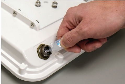
Figure 1.6 – Applying Silicon Dielectric Compound
