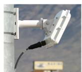
Adjust the side-to-side angle as close to perpendicular to the flow of traffic as possible. This will be fine-tuned later.
