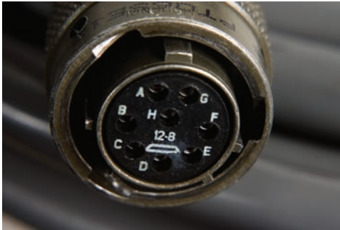
Figure 1.6 - Sensor 6-conductor Cable Connector
