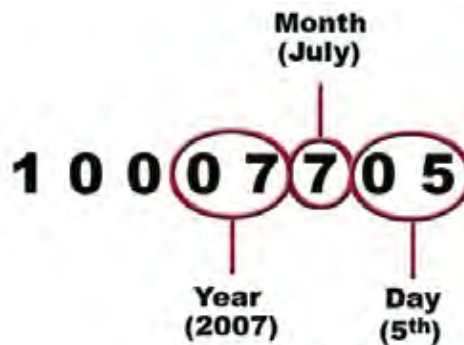
Figure 4.14 - Install Upgrade Numbers
