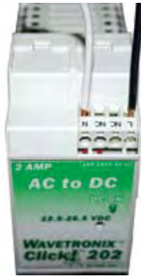
Figure 2.6 - Wiring AC Power into the Click! 201/202
