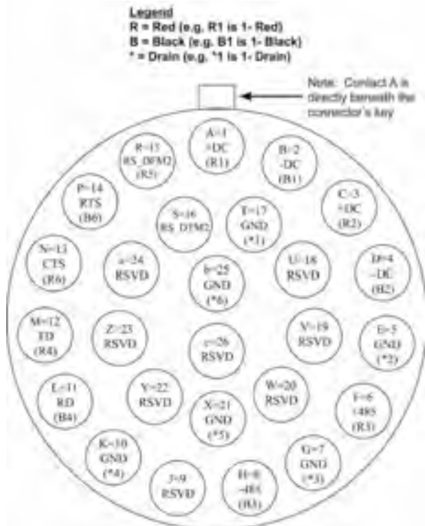
Figure A.3 – Old SmartSensor Plug Connector Socket Assignment as seen from the solder cup side of the connector
