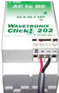
Figure 2.7 - Wiring DC Power Out of the Click! 201/202
