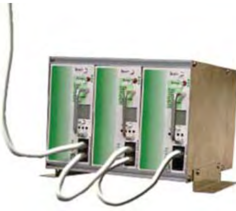
Figure 2.10 – Connecting Contact Closure Modules
