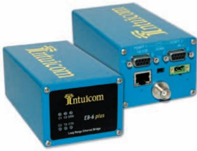
Intuicom's EB-6 PLUS is a long-range, high-speed industrial wireless transceiver enabling both IP and serial connectivity. The EB-6 PLUS provides remote serial and IP data connectivity to IP based networks, enabling high performance data transport, positioning and access for fixed or mobile operations.
