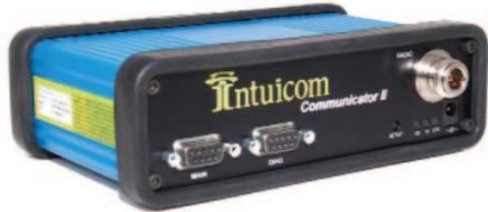
The Communicator II™ is a high performance wireless data transceiver designed for industrial serial and serial to IP networks. The Communicator II enables long-range wireless connectivity at high bandwidths for robust and secure wireless communications for a broad set of fixed and mobile applications.
