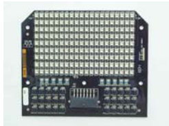
LED array that provides illumination and steerable beam
