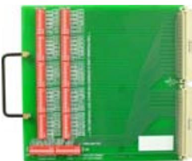
The MMU-EXT Program Card is designed to facilitate cabinet testing when multiple Program Card configurations are needed. DIP switches for all programmable functions of the MMU Program Card make modifications to the MMU set-up fast and easy.
