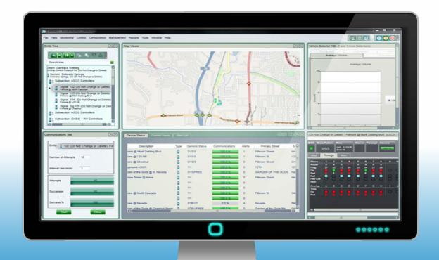
▷ ▷ Centracs MOE module provides these new tools for measuring and assessing factors impacting traffic signal coordination, as well as to satisfy performance measures evaluations.
