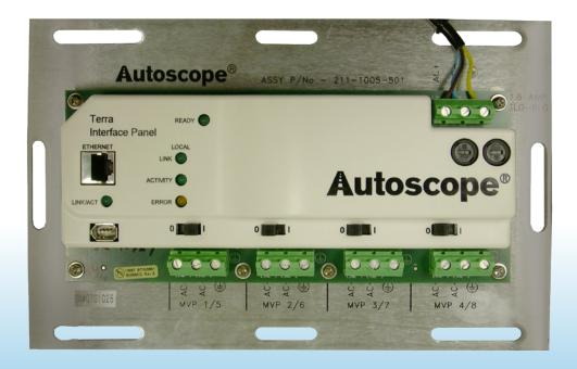
b The Autoscope Interface Panel supports "3-wires-only" branch cable connections to ENCORE detection sensors.
