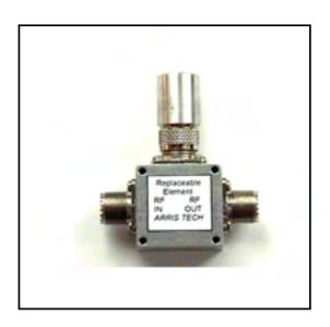
The IMG-UHF is a high performance RF surge suppressor designed to protect high exposure outdoor coaxial signal lines. The IMG-UHF features "PL-259" connectivity IN/Out. Surge suppression is provided by a replaceable solid state cartridge. Field replacements are easily accomplished. Bulkhead/panel mount units are available per special request. Replaceable cartridge – IMG-UHF-C available separately.
