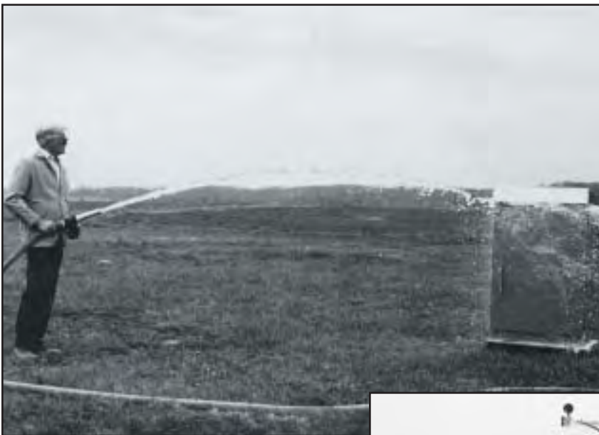
U.L. NEMA 4X - Hose Down Test
