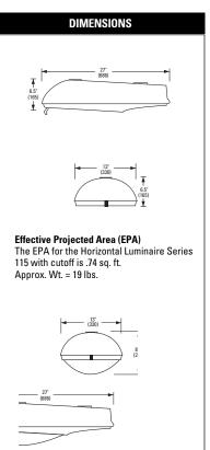
**Effective Projected Area (EPA)** The EPA for the Horizontal Luminaire Series 115 with sag glass is .82 sq. ft.
